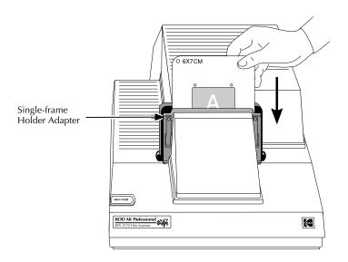
The film holder is now properly inserted into the Scanner.
